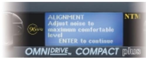
In Alignment Assistant mode, the bands/channels to be measured are chosen. A microphone is used on input C, and pink noise is then automatically output through every band in turn. The FDS-366T will then analyse the signal delays, and automatically adjust the delays to compensate. Field tests have shown this to be not only highly accurate, but the enhancement in image and sound quality is staggering.
