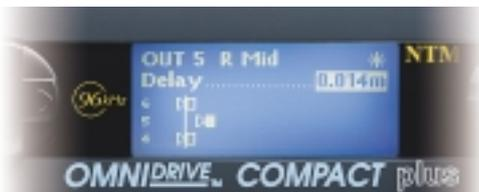
We've always provided highly-accurate delay setting in all our OMNIDRIVE models. The FDS-366T offers precision steps of 10 microseconds on each delay – all 3 inputs and 6 outputs. With a maximum delay setting of 2.6 seconds per channel (including inputs) the FDS-366T can easily compensate for delay towers as well as stereo image correction between stacks, and individual cabinet driver alignments.
