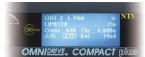
Adjustable Attack and Release speeds are provided (Fast/Medium or Slow) with the speeds ganged to the high-pass crossover frequency for optimal performance depending on the frequency range of the band.
