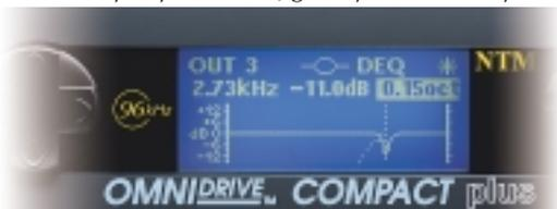
You can determine how much of the program is affected using the bandwidth setting. As an example, consider how some horn drivers can 'bleat' or distort at high levels - using dynamic eq you can cut the offending frequency as the level passes that threshold.
