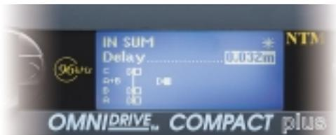
Adjusting the delays is simply a matter of selecting the channel/band, selecting the delay adjust screen and entering the value with the rotary encoder. Delays can be linked and adjusted simultaneously to make correction between different cabinets easily achievable.
