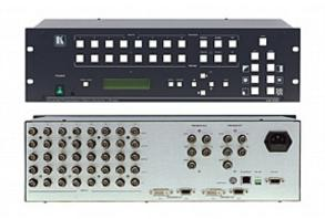
The VP-727 In-CTRL Dual Scaler Seamless Switcher is a true multi-standard video to graphics scaler and seamless switcher with 8 universal inputs comprised of 5 BNCs, any of which can accommodate a composite video, s-Video (Y/C), component video (RGB/YUV), RGBS, or RGBHV signal. It has dual scalers, one for the preview and the other for the program output. Dual scalers are required to do "live" seamless transitions from one source to another.
