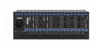
The VS-1616D is a high-performance matrix switcher chassis for AV signals. The unit is modular and populated from 2x2 to 16x16 in increments of two inputs and/or two outputs. The chassis includes a power supply, control module and a test module that can monitor and test any input and output in the matrix. VS-1616D supports a wide variety of input and output cards for different AV signals.
