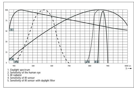
Fig 2.1 Infra-red radiation spectrum in relation to other spectra
