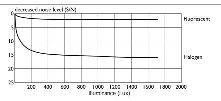
Fig 2.8 S/N ratio decrease when using fluorescent and halogen lighting
