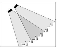
Fig 2.6 Radiator position (in cross-section) in a conference hall with very steep seating.
