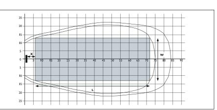
Fig 2.14 A typical radiator footprint for a mounting angle of  $0^{\circ}$ . The shaded rectangle shows the largest rectangular area where the signal-to-noise ratio is at least 40 dB(A). It si this area which is represented in the tables. The length (L), width (W) and horizontal point at which the rectangular footprint starts (X) are shown.
