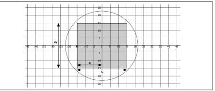
Fig 2.15 A typical radiator footprint for a mounting angle of 90°. X is negative because the radiator is actually mounted beyond the horizontal point at which the rectangular footprint starts.
