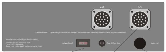
Mains power inlet on 1.5M flying lead terminated with a 5 pole 32A ceetype cable plug
