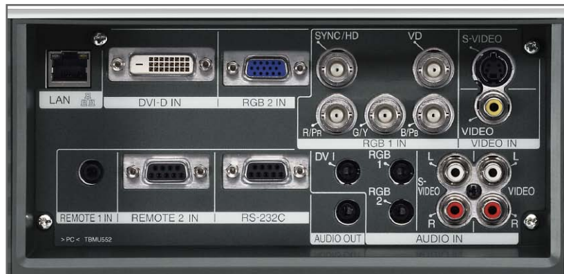
Terminals include an HDCP-compliant DVI-D input connector
