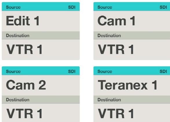
In this example, the scroll wheel is being used to list all sources that can be routed to the destination VTR 1, based upon the SDI routing level. When the scroll wheel is rotated, the names of source equipment are progressively displayed to make it very easy to find the desired video source.
