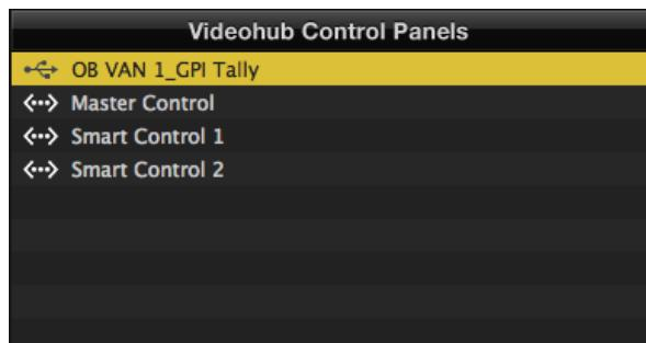
GPI and Tally Interface connected via USB.
