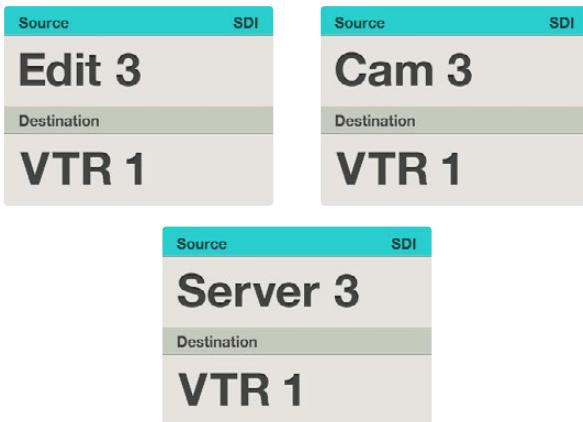
In this example, the numeric button "3" has been selected so only video sources with a "3" in their label will be listed, on the LCD, when the scroll wheel is rotated. This provides a fast way to find a video source because you only have to scroll through a short list of equipment based upon a group number, e.g. only list the equipment in Studio 3.
