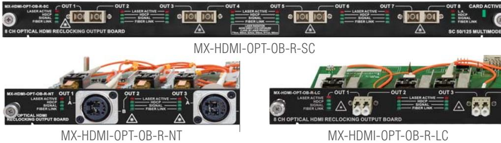
MX-HDMI-3D-OB-R is an eight channel Multimode optical Output Board providing HDMI 1.4, audio and RS-232 extension over a single Multimode fiber up to 2500m distance. Pixel Accurate Reclocking, HDCP compliance and HDMI to DVI conversion are incorporated. Resolutions up to 4K and 36-bit color depth are handled with all standard audio formats as well as 120Hz 3D signals.
